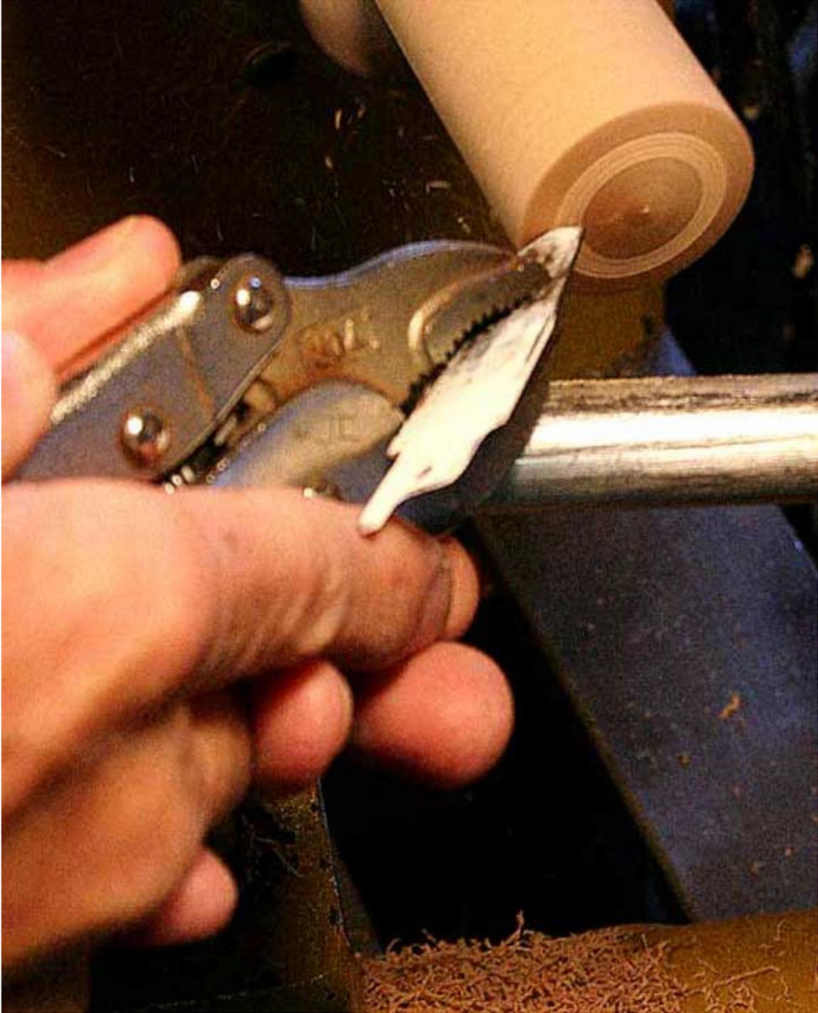
This is the chatter tool in use. Move the tool rest back about 2". You want the vise grips on the tool rest. You may need to lower it also. For your first experiments position the tool so it cuts about 7 to 8 o'clock and tilted down like using a scraper. You can tilt the tool to the left, the right or straight up. There are a lot of variables to chatter work so you must be willing to experiment.
