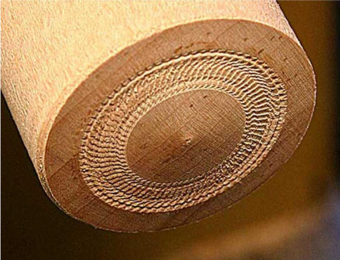
This is an example of the chatter work this tool will do on maple end grain. Below is a sample of some of the chatter work I've done on Corian, Tagua Nut, and cocobolo. If you look at the Cocobolo piece you will see that the chatter work angles in two different directions. This is what happens when you tilt the tool left for one cut and then right for another. I cleaned up the joint where the meet with my spindle gouge as well as the outer edges.
