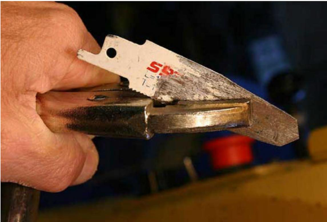
To use the tool simply clamp it in a pair of vise grips. Extend the tip out about an inch. More extension makes the tool vibrate slower. Less extension makes it vibrate faster. The faster it vibrates the closer the chatter work marks are together.
