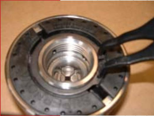
Position backing plate to pinions like in picture and push down so that the plastic backing plate is flat with the chuck.
