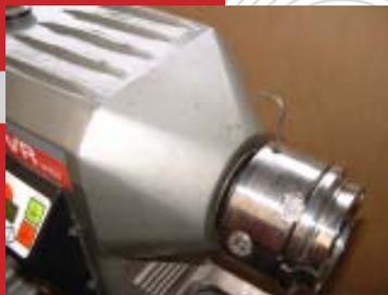
Using the 3mm Allen key provided with the Supernova release M6 grub screw (turning anti-clock wise direction to loosen)
