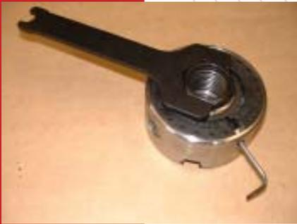
Using 1/2" spanner wind the insert back in, make sure the spigot is in full contact with the back of the chuck. This is important for accuracy. Once insert is fully engaged screw in M6 grub screw with 3mm Allen key provided.
