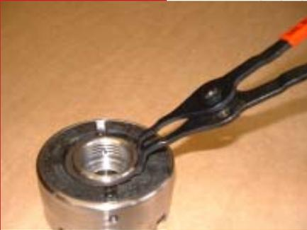
Using circlip pliers remove circlip from bottom of chuck holding in the plastic backing. **YOU MUST WEAR SAFTEY GLASSES WHILE PERFORMING THIS OPERATION AS CIRCLIP MAY FLY UPWARDS OFF PLIERS**
