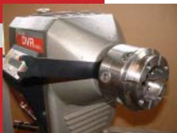
Using a ½" spanner (like accessory 23014 pictured) undo the insert from the lathe. Make sure the spindle lock on the lathe is engaged and hit the spanner with a block of wood or plastic mallet in an anti-clock wise direction
