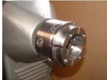
The Supernova 2 chuck on Nova 3000 DVR lathe
