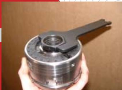
With the chuck in your hand and using the ½" spanner again hit the spanner with a block of wood or plastic mallet is disengage the insert from the chuck
