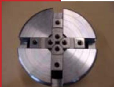
Push all jaw slides to meet in center forming a square. There is no starting slide way so you may choose any one. Starting with Jawslide 1 insert jaws in clockwise direction in numerical order.
