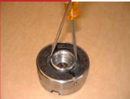
Using two flat head screw drivers gently push together to lift both sides evenly. Do not try to force out straight away as this may damage plastic, work on bringing both sides up together at the same time. Remove plastic backing completely exposing pinions and back of scroll ring.
