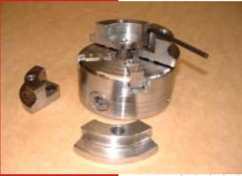
With the 4mm allen key provided release all jaws from the chuck by un screwing the M6 conuter sunk screws
