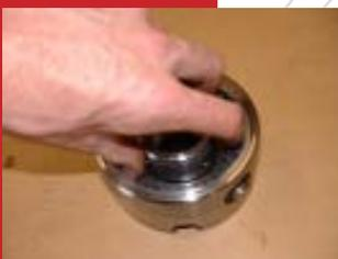
Place scroll ring in chuck and move it back with your fingers as demonstrated in the picture. You will know once it has engaged as it will drop down allowing the pinions to fit in. Make sure the jaws have not moved and still have a square formed in the centre.
